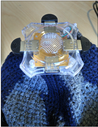
Figure 4: Our prototype with 3 USB mini-microphones, attached to a 4-port USB hub.
